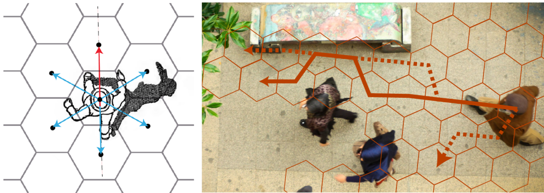
Figure 10: Example of Honeycomb walking pedestrian behavior model
