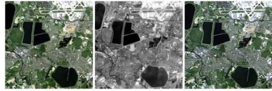
Fig. 5 Examples of Image Fusion in remote sensing domain. (a) noise free MS image (b) PAN image (c) Fused image.
