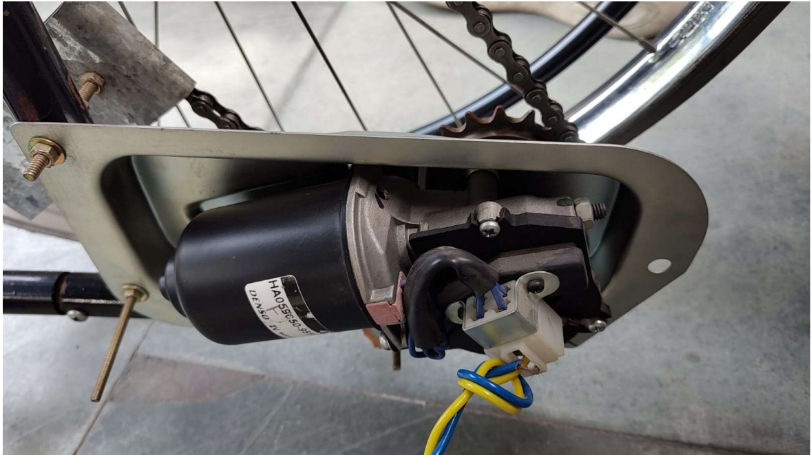
Fig. 2 Viper Motor fitted in the chassis rod by drilling out the chassis rod and passing a nut-bolt (M3*12 mm)
