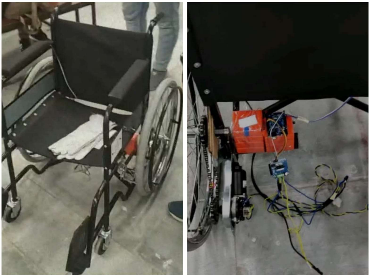
Fig. 14 Final prototype: Fully assembled wheelchair capable of being operated solely through hand gestures.
