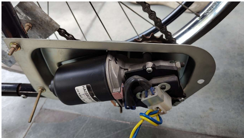
Fig. 8 DC Viper Motor (14W, 12V)
