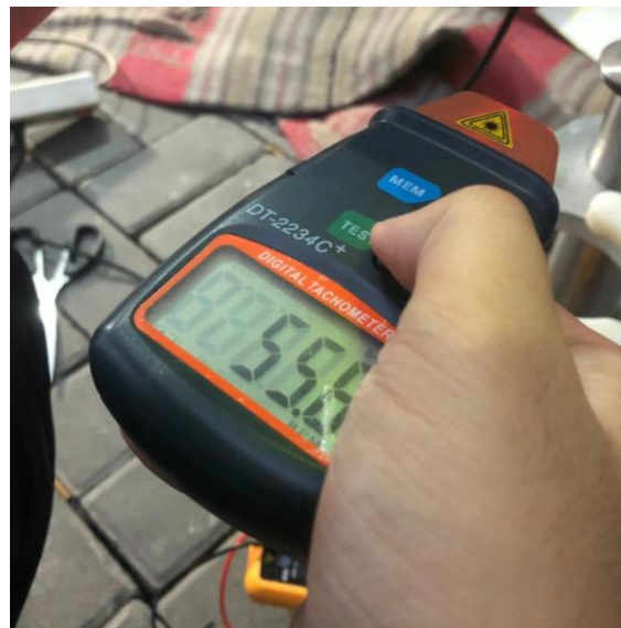
Figure 15. Testing dc motor rpm with tachometer
