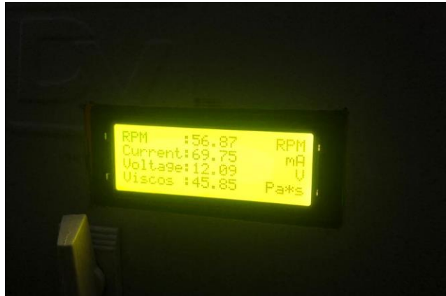
Figure 14. Speed sensor test (optocoupler fc 03)
