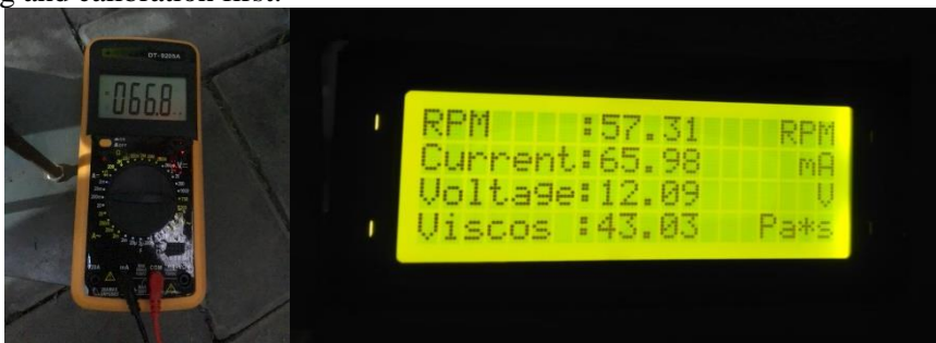
Figure 10. DC motor current test
