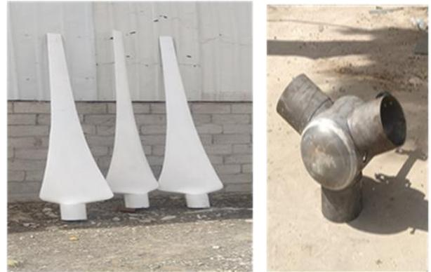
Fig. 11. Final shape of the blades and hub after completing the manufacturing process.
