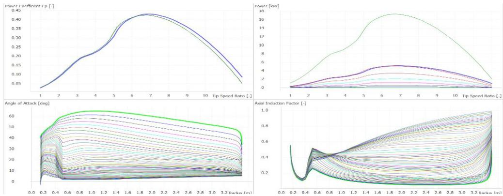
Fig. 4. The simulation results for the airfoil shape of the blade
