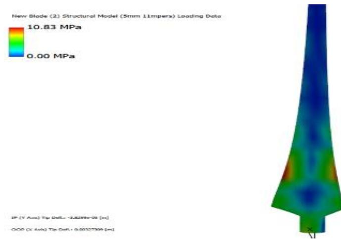
Fig. 5. Displays the corresponding results for the loads acting on each part of the blade at a wind speed of 11 m/s and a thickness of 0.5 cm
