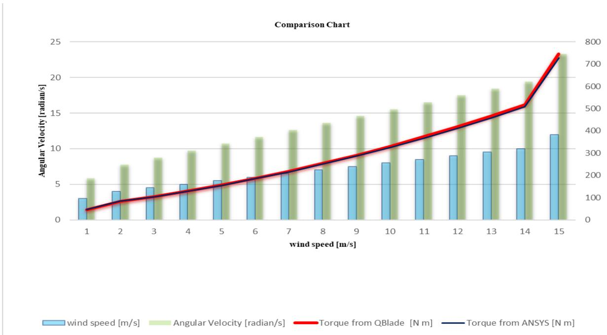
Fig. 7. torque results compared for various wind speeds and rotational velocities.
