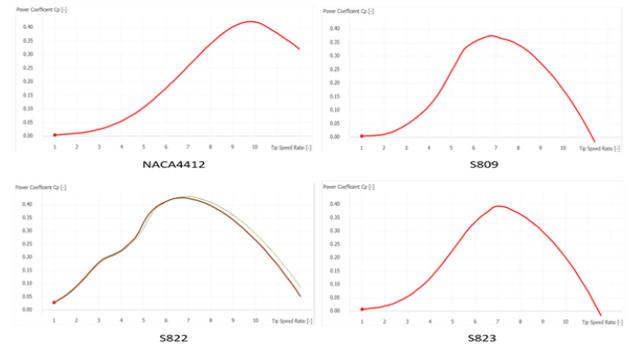
Fig. 3. Cp values for each type of tested airfoil surface
