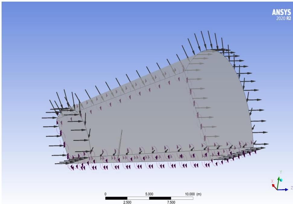
Fig. 6. CFX tool to define boundary conditions and other parameters
