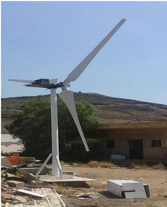
Fig. 13. The blades after being installed on the test tower
