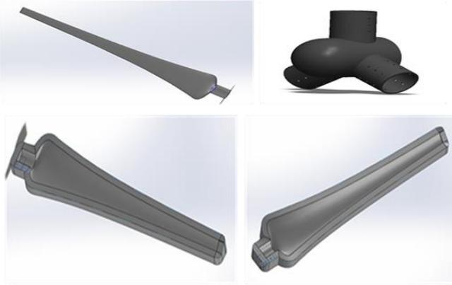
Fig. 8. The mold, blades, and Hub in SOLIDWORKS.
