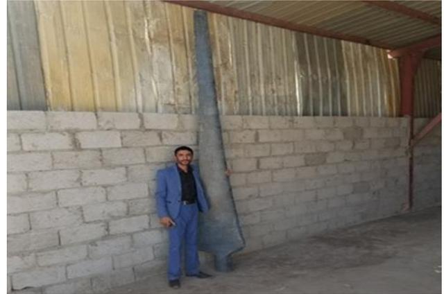
Fig. 10. The shape of the blade obtained after the completion of the infusion process.
