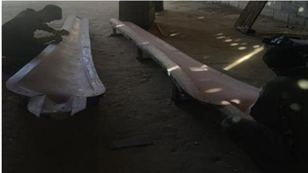
Fig. 9. The mold for the blades after it has been prepared.
