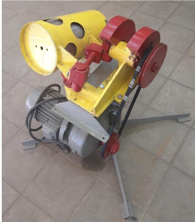
Fig. 1. The main elements of the experimental installation of the mixer are the mixer support, stand, electric motor, gearbox, four-link mechanism, mixing tank.
