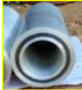
Fig. 4. The sandwich pipe structures AA-AA-HDPE.
