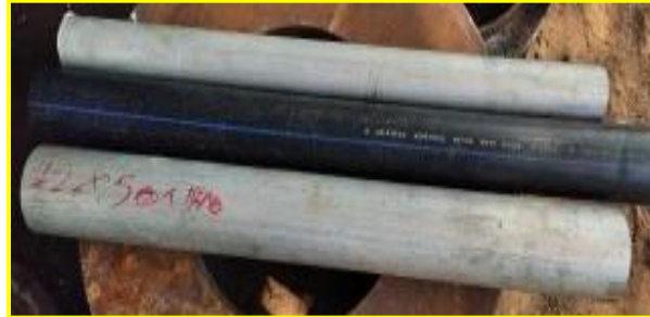
Fig. 2. The sandwich pipe of aluminium, HDPE, and aluminium materials.
