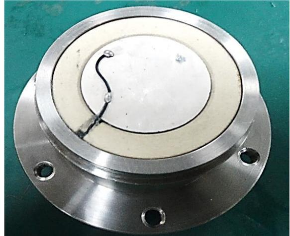
Figure 4 Echo sounder prototype before molding
