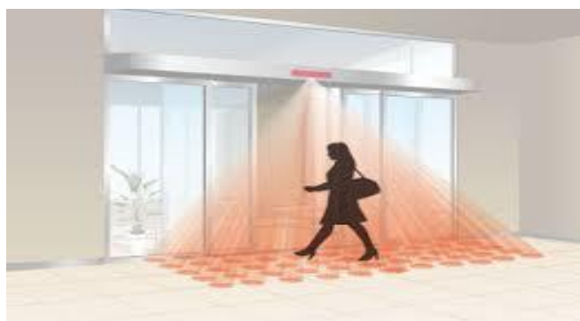
Fig 2.0 A censoring door which detect the person in front of him and open Automatically with the help of sensors.
