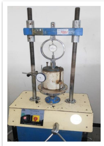
Fig. 2. PET bottle cell with infill material installation in CBR mould. Fig. 3. California Bearing Ratio Test Set up.
