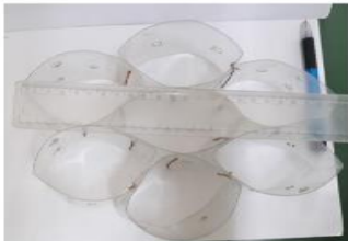
Fig(d): PET bottle geocell
